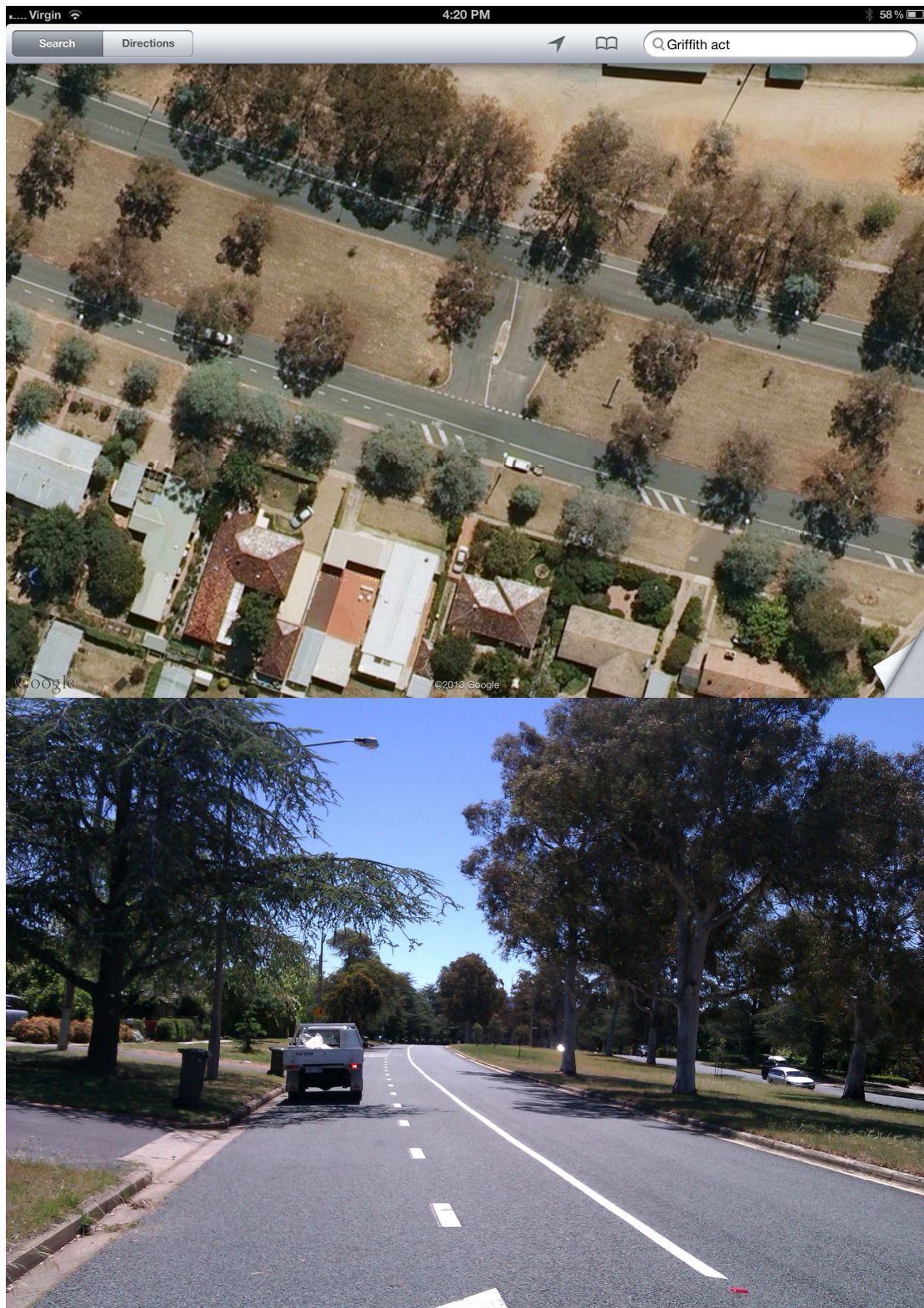
Figure 13: Cycle lane occupies part of the parking ‘door zone’ of the parking lane. (Northbound carriageway, Captain Cook Crescent)
